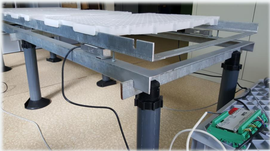
4 single load cells in between 2 steel frames and transmitterbox
